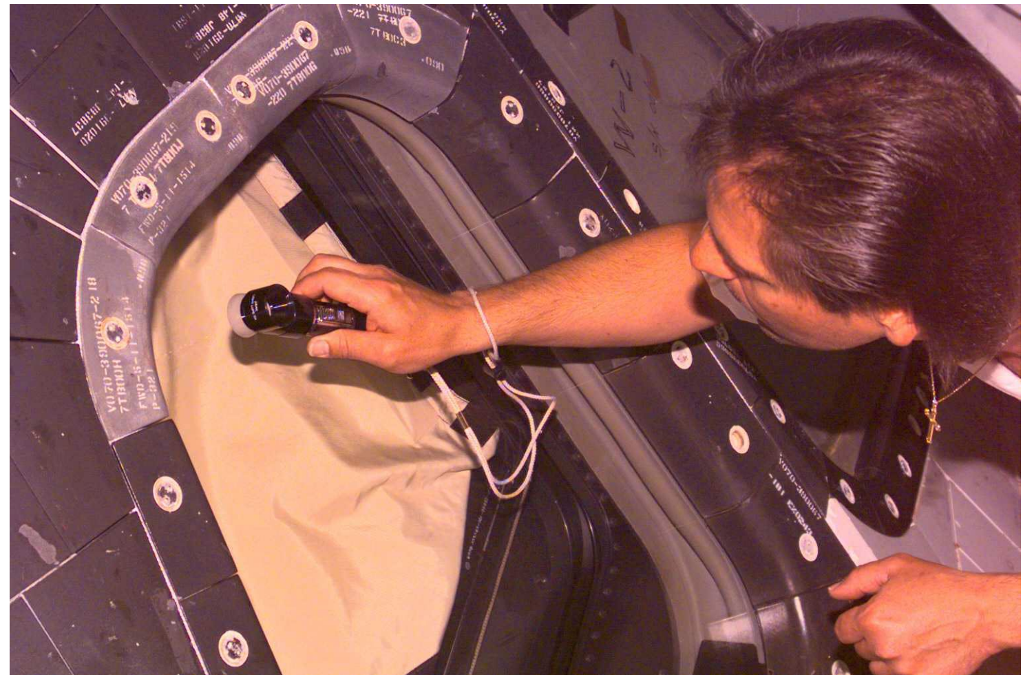
Space Shuttle window being inspected for orbital debris impacts
